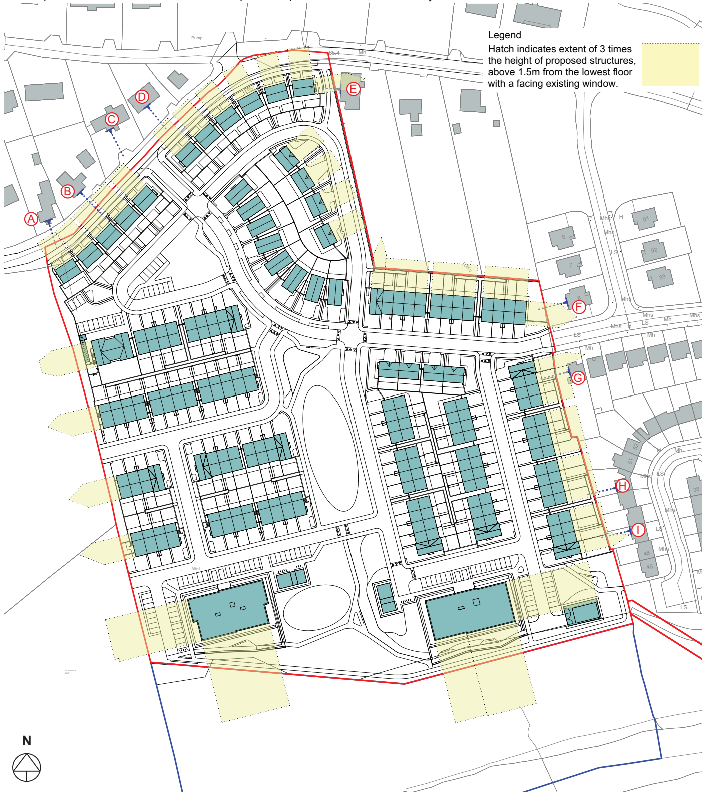
Figure 2: Proposed site plan showing the zone of influence from the proposed building and direction of the window wall of neighbouring residential properties.
